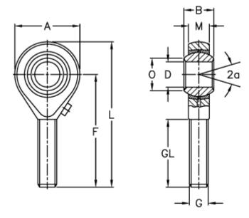
$\begin{array}{lll} A & = 60 \\ a \text{ (degrees)} & = 15 \\ B & = 31 \\ D & = 25 \\ Dynamic load C \text{ (kN)} = 40.5 \\ F & = 94 \\ g & = M24x2 \\ GL & = 57 \\ \end{array}$
